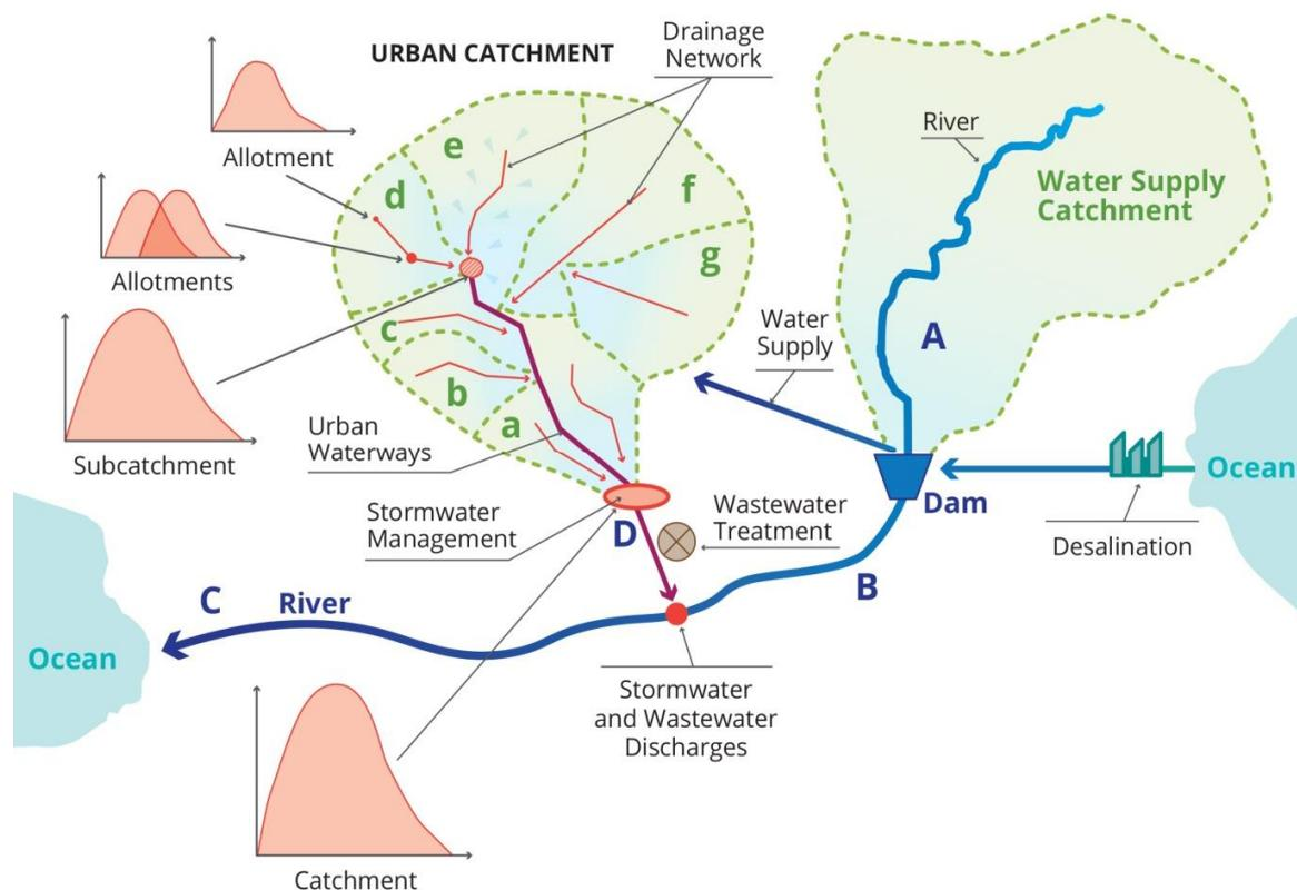
**Figure 1: Schematic of traditional urban catchments and cumulative stormwater runoff processes**
