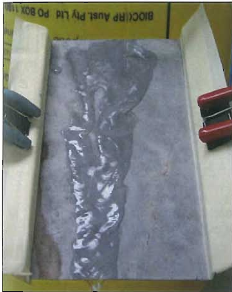
Figure 4-3: Determination of lead mobilisation off heavily oxidised flashing from slow flow (0.4L/min) runoff
