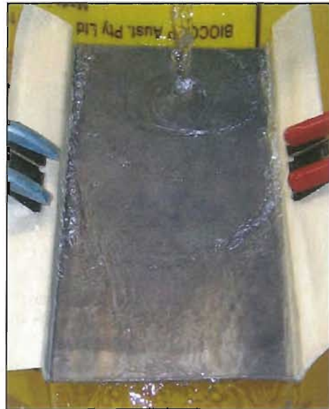
Figure 4-4: Determination of lead mobilisation off new un-oxidised lead flashing from fast flow (5.5L/min) runoff
