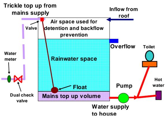
Figure 3: Design of the dual water supply system
